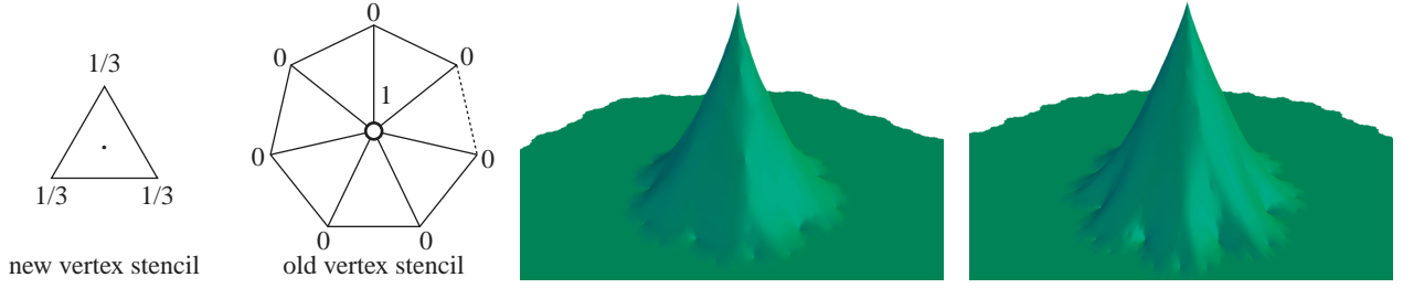
Figure 2: The simplest primal \sqrt{3} -subdivision scheme computes new control points which correspond to faces on the coarser level by averaging all incident triangle vertex control points (left). Control points for vertices inherited from the coarser mesh are copies of control points from the old mesh. Because of the latter the resulting scheme is interpolating. Examples of basis functions in the regular respectively irregular (valence 9) setting are shown on the right.
