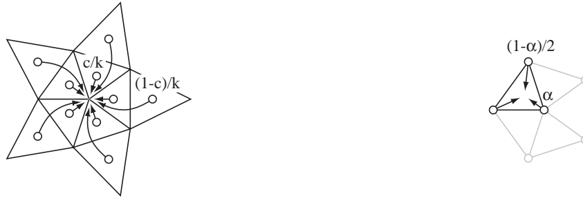
(a) Flap modification FV_c at an irregular vertex as a function of the parameter c .
