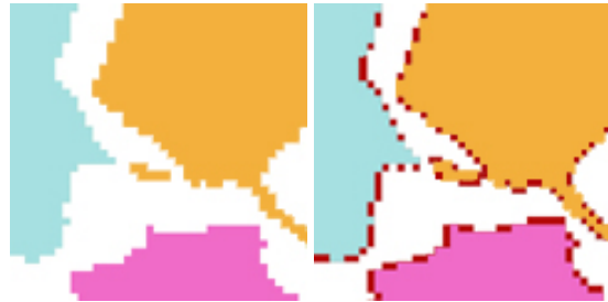
Figure 5: Rasterizing the boundary of the chart ensures that it is connected. (Samples in red are added by boundary rasterization.)
