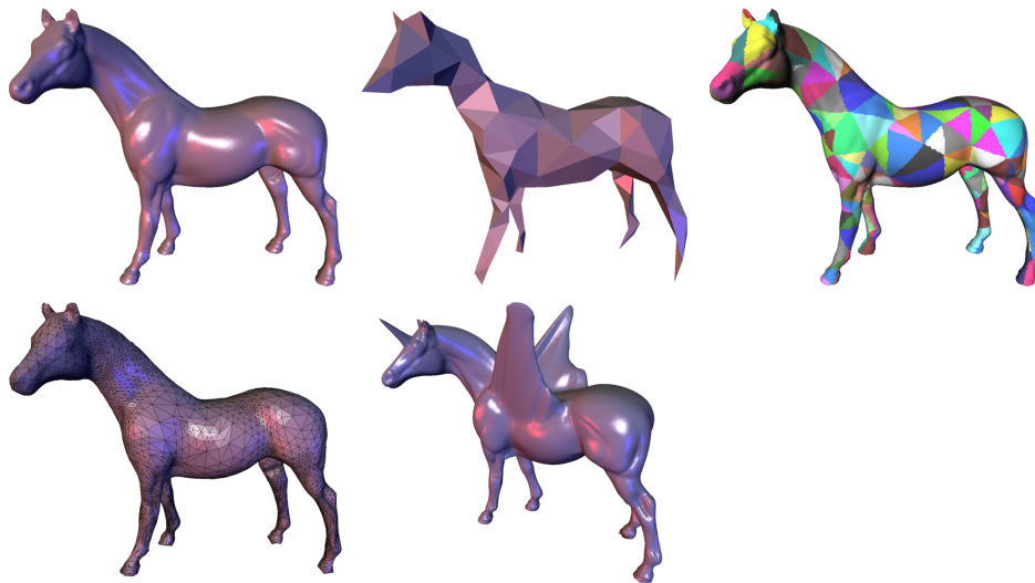
Fig. 1.15. Overview of the remeshing algorithm. Top left: a scanned input mesh (courtesy Cyberware). Next the parameter or base domain, obtained through mesh simplification. Top right: regions of the original mesh colored according to their assigned base domain triangle. Bottom left: adaptive remeshing with subdivision connectivity ( \epsilon = 1\% ). Bottom middle: multiresolution edit.
