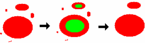
Removing Noisy Objects by Contracting then Expanding the Distance Function
