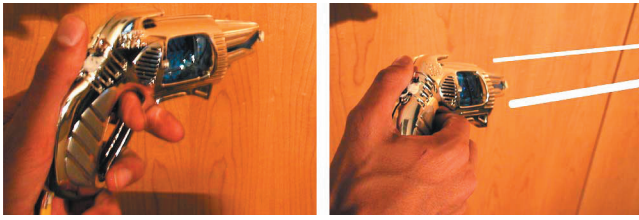
Figure 8: The raygun tool: Pressing the menu button (right) displays the two current options for the gun: drawing Phosphate bonds (thin line) and drawing Hydrogen bonds.
