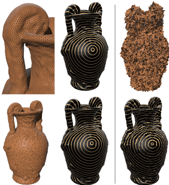
Fig. 16. Tests of robustness. Left: our smoothed distance ( m = 10^4 ) appears similar on meshes of different resolution. Right: even for meshes with severe noise (top) we recover a good approximation of the distance function on the original surface (bottom, visualized on noise-free mesh).
