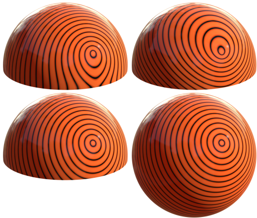
Fig. 11. Effect of Neumann (top-left), Dirichlet (top-right) and averaged (bottom-left) boundary conditions on smoothed distance. Averaged boundary conditions mimic the behavior of the same surface without boundary.
